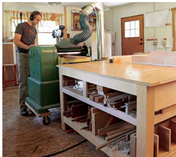
Ambidextrous outfeed table. Korsak situated his tablesaw and planer so they share a single outfeed table, which also serves as an assembly table. A shopmade mobile base elevates the planer to make the shared outfeed possible.
