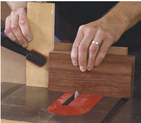
Canted kerf. The base joinery begins with a kerf cut in the foot blank at 45° for the gunstock miter.
