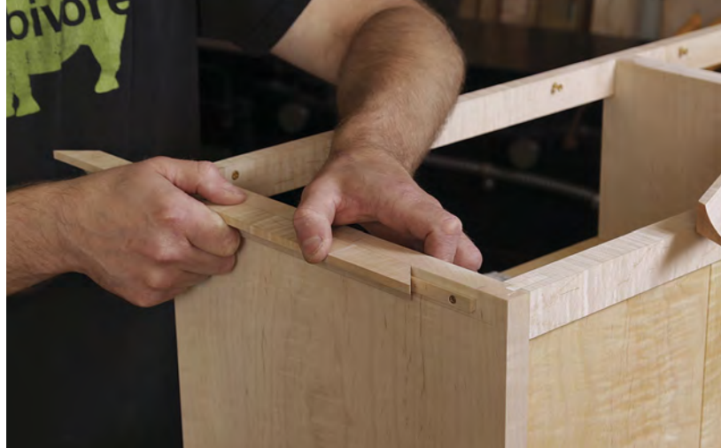
Slide on the side molding. Having already cut and fitted the front miters on the side molding, Korsak unscrews the front molding and slides the side molding onto the cleat to mark for the rear miters.
