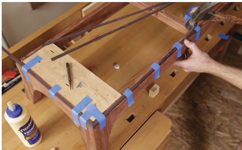
Glue the beads into the rabbet. Korsak uses painter's tape to keep the beads in place as he fixes them with glue and brads.
