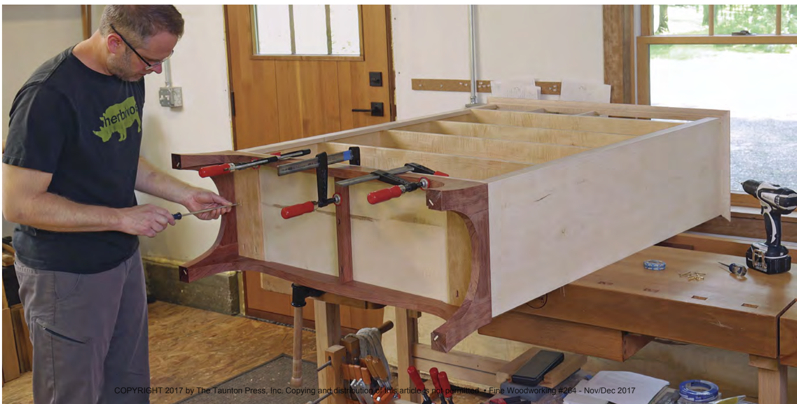
Screws keep the base in place. Elongated clearance holes permit the case to move with the seasons.
