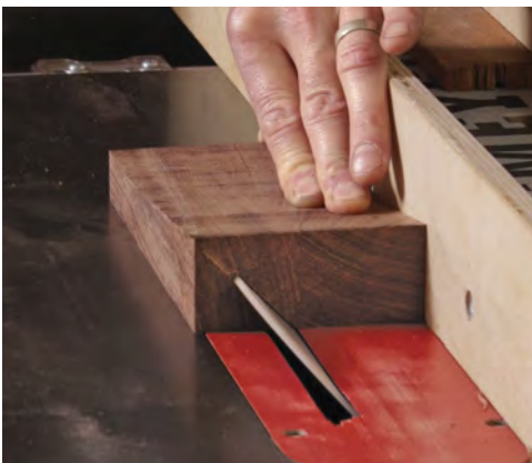
The feet meet in a miter. Korsak miters the feet at the tablesaw, cutting in several passes to reduce pressure on the short workpiece.
