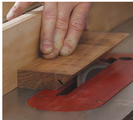
Slot for a spline. With the feet mitered and the fence moved to the other side of the blade, cut a groove for the spline.
