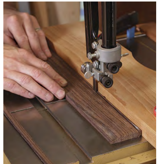
Slit into strips. Cut the beads free at the bandsaw, then smooth the bandsawn face of the bead with a handplane.
