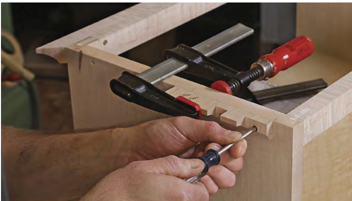
Invaluable scrap. A piece of scrap molding with a dovetail socket guides attachment of the cleat. Clamp the scrap flush to the top of the case, slide the cleat into the socket, and drill and screw it into place.
