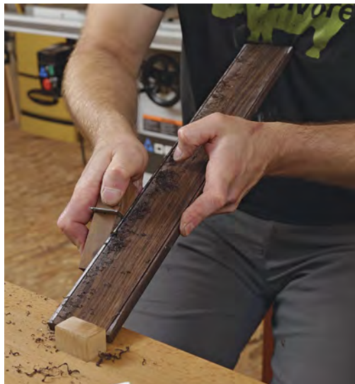
Beads by hand. With a shopmade scratch stock, Korsak cuts beads on both edges of a wide rosewood workpiece.
