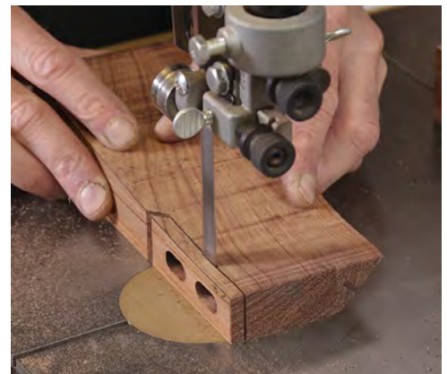
Finish the gunstock. Korsak roughs out the shoulder on the bandsaw. He'll follow up with multiple crosscuts on the tablesaw.
