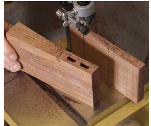
Bandsaw the sweep. The face of the foot is bandsawn to a curve.
