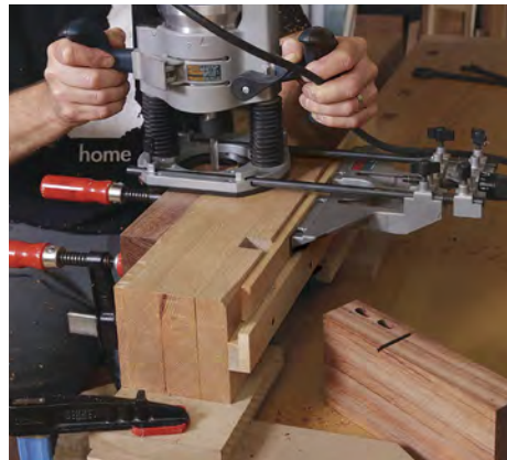
Sliding jig for slip tenons. Korsak made a router jig that has a channel on the back that captures the router fence, steadying the cut.
