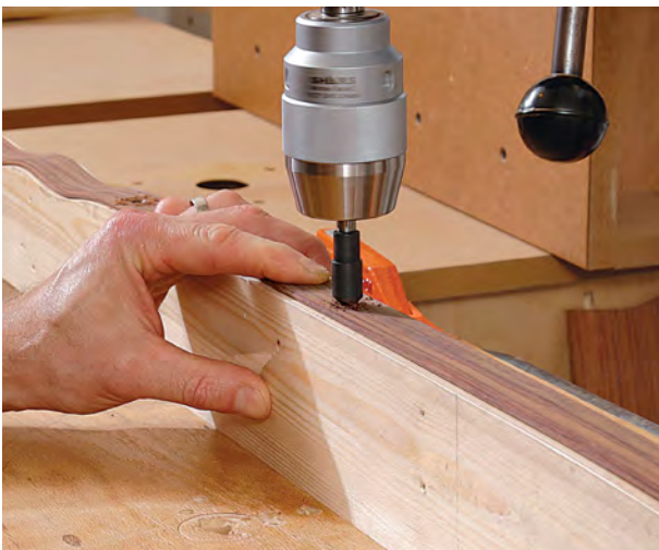
Prepare for attachment. Korsak countersinks the bead for screws that will keep it from shifting during glue-up. He ebonized the bead with leather dye, then applied shellac.
