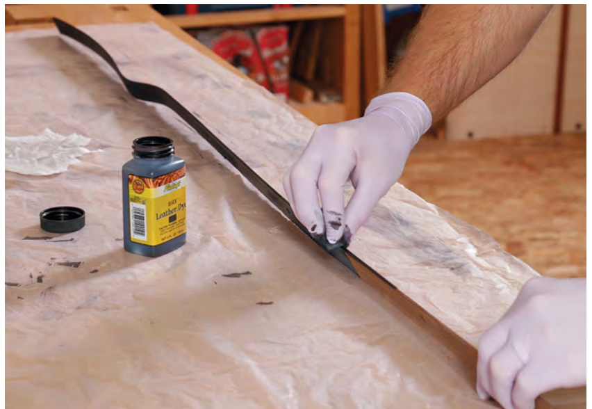
Prepare for attachment. Korsak countersinks the bead for screws that will keep it from shifting during glue-up. He ebonized the bead with leather dye, then applied shellac.
